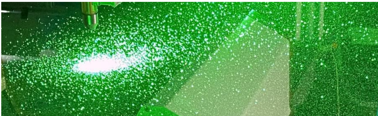
Figure 1. Laser Sheet Imaging of an electrostatic-assisted air-atomizing spray nozzle
